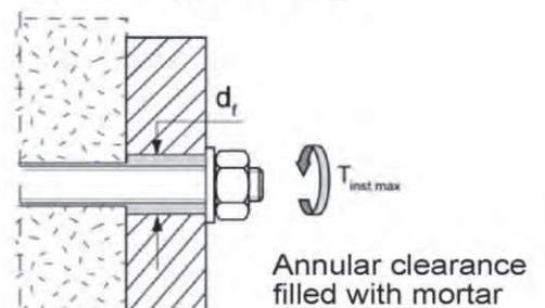
**Internal threaded anchors UPM-I without perforated sleeve UPM SH K; installation in solid brick masonry and autoclaved aerated concrete**
