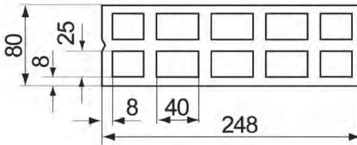
Table C68: Installation parameters for threaded rod with perforated sleeve
