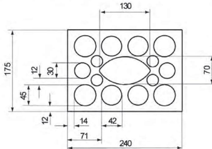
Table C32: Installation parameters for threaded rod with perforated sleeve and internal threaded anchor UPM-I with perforated sleeve
