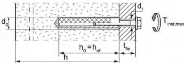
**Threaded rods and internal threaded anchors UPM-I without perforated sleeve UPM SH K; installation in autoclaved aerated concrete (installation with special conic drill bit PBB)**
